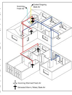
The system is designed to run continuously and should NOT be switched off except for maintenance or filter replacement. It is important to follow the advice in this user manual and correctly install and maintain the system to ensure a healthy and comfortable indoor environment.
